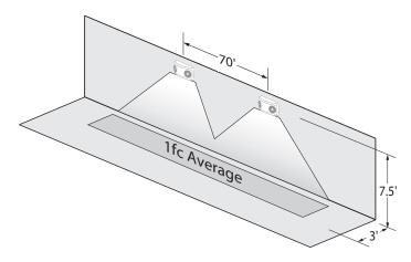
Using multiple NFT units (2.7 Watts lamps) mounted at a typical 7.5' height delivers 63' on center spacing with a 6' wide path of egress.
