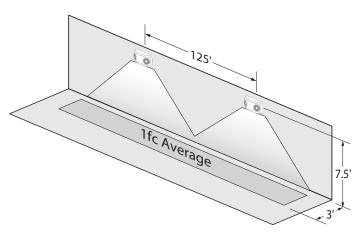
Using multiple NFT-HO units (5.4 Watts lamps) mounted at a typical 7.5' height delivers 115' on center spacing with a 6' wide path of egress.
